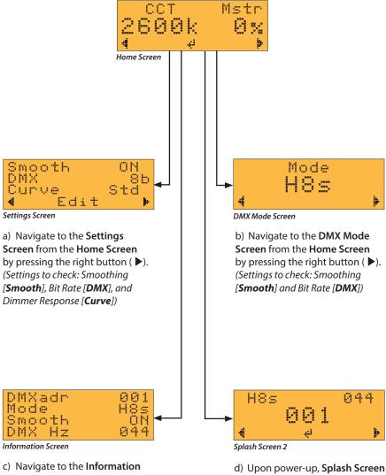
C) Navigate to the Information Screen, which is only a splash screen (i.e., it automatically times out), from the Home Screen by pressing the center button. (Settings to check: Smoothing [Smooth] and Bit Rate [DMX]) d) Upon power-up, **Splash Screen** 2 (which appears immediately before the **Home Screen**) will display settings before timing out. (*Settings to check: Smoothing* [**Smooth**] and Bit Rate [**DMX**])
